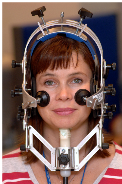
Figure 1 Headset to hold probe steady and allow natural head movement during speech. Despite resembling a constraining medical device, the headset feels like a sports helmet and was generally regarded by subjects as amusing and “cool”.
